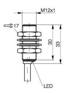
**Inductive Sensors** BES 516-375-E4-C-03 M12x1 x 33 normally-closed Sn=2mm shielded
